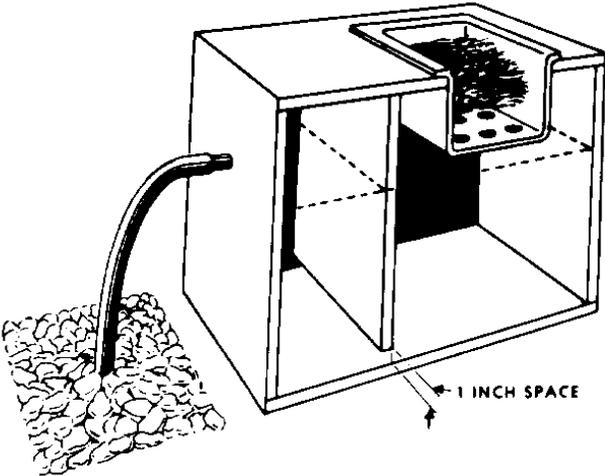
Figure 5-4. Grease trap.
