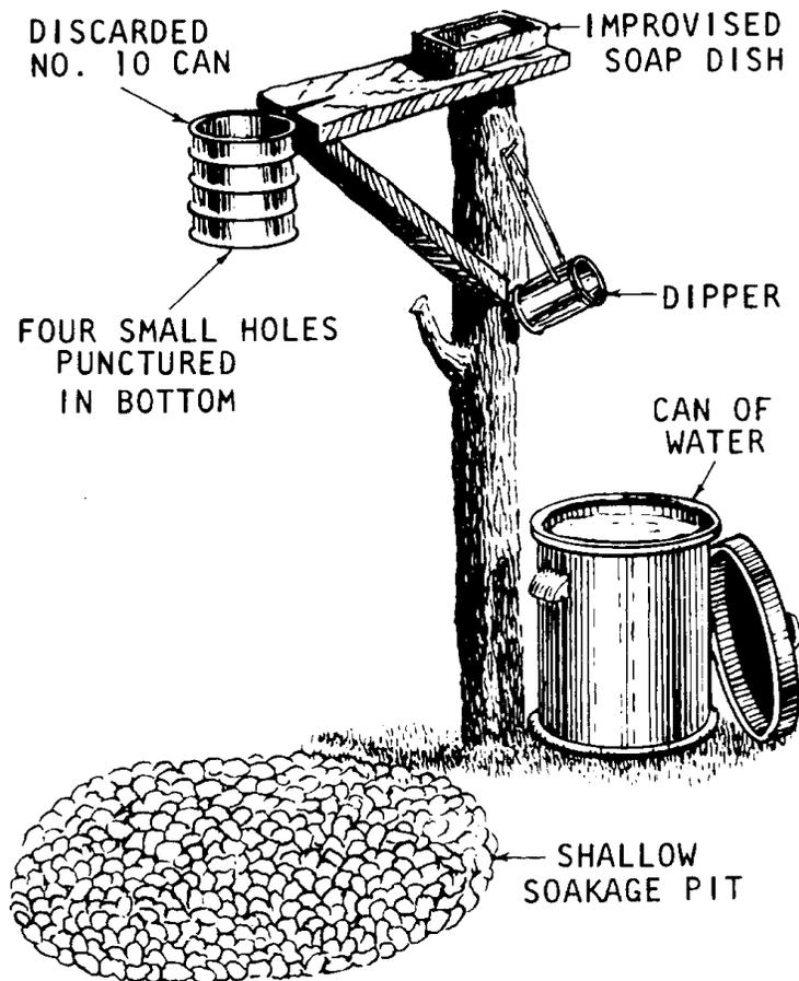
Figure 5-10. Handwashing device.
