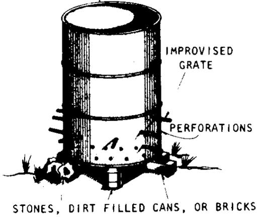
Figure 5-2. Grate incinerator.
